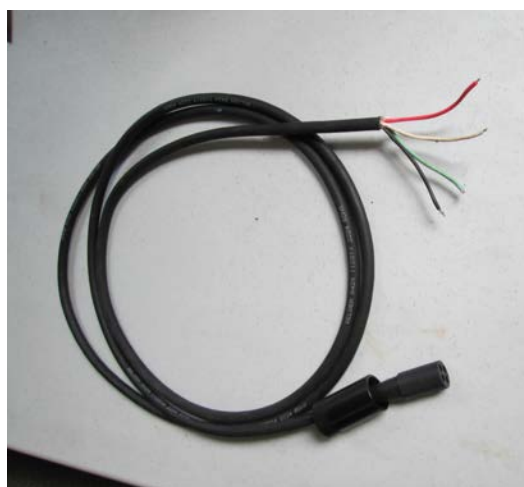
Underwater pigtailed cable with connector and locking sleeve
