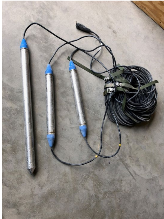
FIGURE E.I-5. BOREHOLE GEOPHONE AND GNSS SYSTEMS
